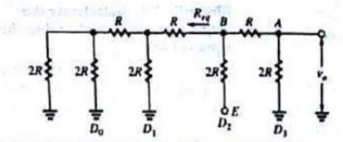
(a) When the input is 0100, D<sub>0</sub>, D<sub>1</sub>, and D<sub>1</sub> are grounded and D<sub>2</sub> is E volts.
