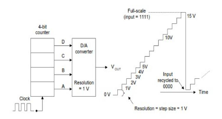
Fig. 7.3 : Output wave forms of a four bit DAC.
