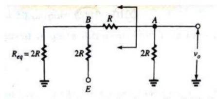
(b) The circuit equivalent to (a) when the network to the left of node B is replaced by its equivalent resistance (2R). The Thevenin equivalent circuit to the left of the bracketed arrows is shown in (c).
